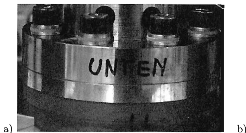
Figure 5.5: Electrical isolation of the specimen: a) plastic isolation disc, b) electrical isolation of the screw
