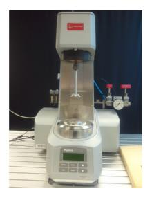
Figure 4.1: The Physica MCR 301 rheometer with plate-plate device
