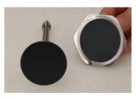
Figure 5.5: Flow curve test of liquid foam by using smooth plate-plate geometry and rough plate-plate geometry (with sandpaper P320).
